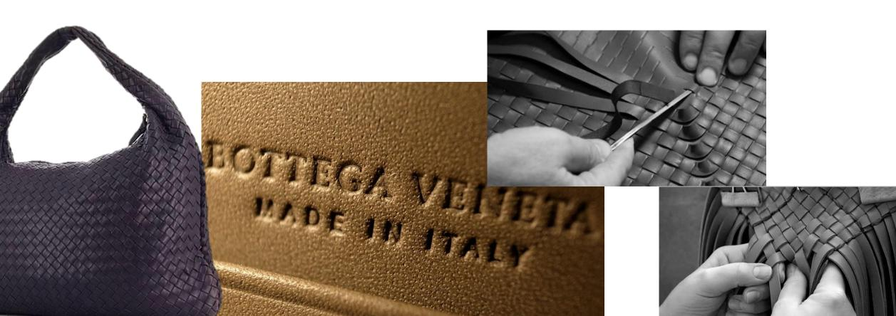
The art of weaving invented by Bottega Veneta. It consists in intertwining strips of leather, following a very precise design, to create a real fabric. It is an artisanal technique in which a lot of manual force and two people are needed to create a meter and a half of processed product
